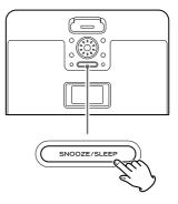
After the ON time is reached, press the SNOOZE button repeatedly to select the temporary turn off time.
